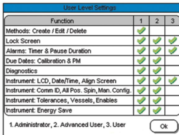
**User access levels** – Control access and eliminate entry errors by placing the 708-DS in a specific mode that prohibits the execution of certain functions.
