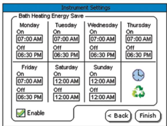
**Heater/Circulator Energy Save** – Program on/off times for your 708-DS heater/circulator to minimize power use; simply enter the desired schedule to ready your apparatus for use.
